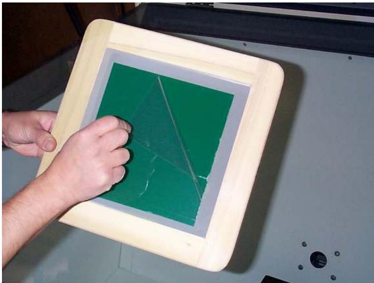
In less than 30 minutes from when you degreased, you will know when the stencil is dry when the backing sheet pulls off easily with very little sound (no tug or crackling sound). Remember to pull off the backing sheet before you tape a positive to the stencil for exposure.
