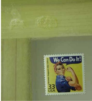
The principle behind capillary film is to barely wet the surface of the film so it sticks to the mesh. We wet the mesh and the film (capillary action) absorbs that water and the film softens and sticks to the mesh. Think of a postage stamp that sticks when you get it wet, only you wet the envelope and that moisture wets the stamp, which makes it stick.
