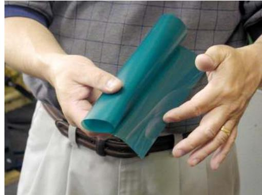
Capillary film is desirable because you don't have to wait until the screen is dry like you do with liquid emulsion, you always have a super smooth surface, always the same thickness, ready to expose stencil in less than 30 minutes.
